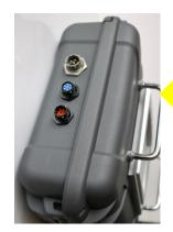
Data logger left side showing power connection (3 pin), flow connection, and discharge pressure connection.
