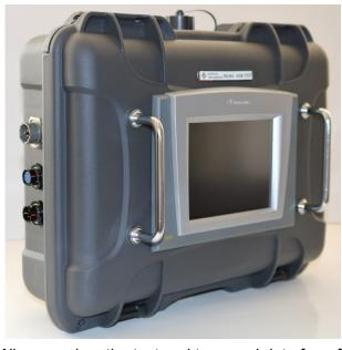
This data logger receives data from three thermocouples, one frequency signal and one analog 4-20 milliamp transmitter.
