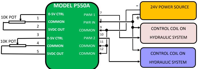
THE INPUT 0-5V CONTROL VOLTAGE MAY BE DEVELOPED WITH A POT AS SHOWN,
