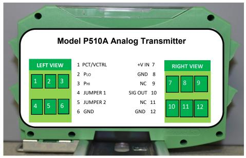
USING A POTIOMETER INPUT AS SHOWN BELOW, THE OUTPUT IS 4-20 MILLIAMPS.
